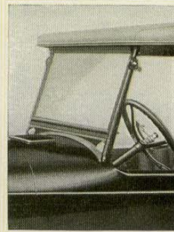
The one-piece, rain-proof windshield provides clear vision. Cowl ventilator. Attractive cowl lights in the windshield base.
