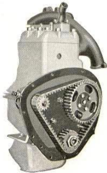
The timing gears are driven by silent chain; lubricated by oil pumped from crankcase; accessible outside adjustment.
