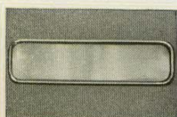
The one-piece rear curtain (no seams) carries a large rectangular glass window which is bound by an enameled moulding.
