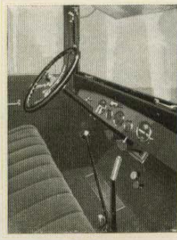
The long gear shift and emergency brake levers are within easy reach of the driver, as are the other controls and the instrument board.
