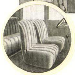
The auxiliary seat, identical in design and cushioning with the driver's seat, folds out of the way when not in use.
